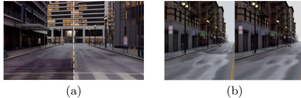
Fig. 3. (a) Resample (left) vs. AGInpaint (right): AGInpaint inpaints slim regions more faithfully. (b) Without (left) and with (right) GCAAlign: GCAAlign harmonizes the seams caused by exposure differences.
